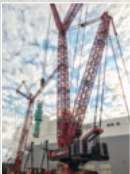
The Big Lift, 1350 Ton Liebherr 11350 Crane with load capacity of 252,827 kilograms at 61.5 metre radius.
