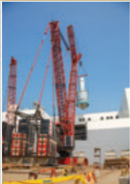
The Big Lift, 1350 Ton Liebherr 11350 Crane with load capacity of 252,827 kilograms at 61.5 metre radius.
