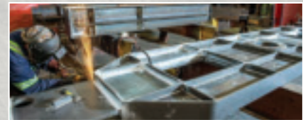
Fabricator Owen Doy grinds to prepare for a weld on a massive equalizer frame for a theme park attraction.
